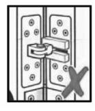
Installing the closer the wrong way will result in failure and is not covered by the manufactures warranty or guarantee.
