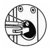
To safely hold the door in an open position where it is possible to fix the closer in place. The closer is supplied with a retaining plate. Care should be taken when inserting the closer to ensure the plate is accessible, but at no risk of being knocked off, as the force of the spring in the closer may cause injury.
